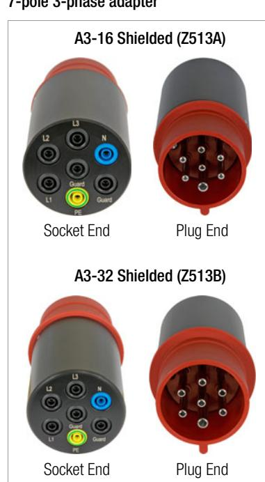
Shielded A3-16 and A3-32 three-phase adapters are used for trouble-free connection of test instruments to 7-pole CEE outlets. The two variants differ with regard to plug size, which corresponds respectively to 7-pole CEE outlets with current ratings of 16 and 32 A.
