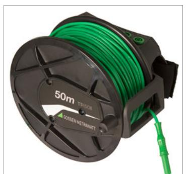
50 m measurement cable coiled onto a plastic reel. Connection to the inside end of the cable is made possible with two sockets integrated into the reel. The other end is equipped with a banana plug.
