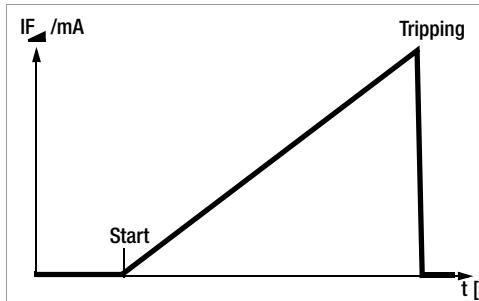
With the selector switch in the  $I_F$  position, slowly rising DC current flows via N and PE. The momentary measured current value is continuously displayed. When the RCCB is tripped, the last measured current value is displayed. A greatly reduced rate of increase is used for delayed RCCBs (type
