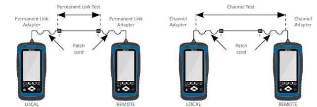
Press the **[AUTOTEST]** button to perform a certification test.
